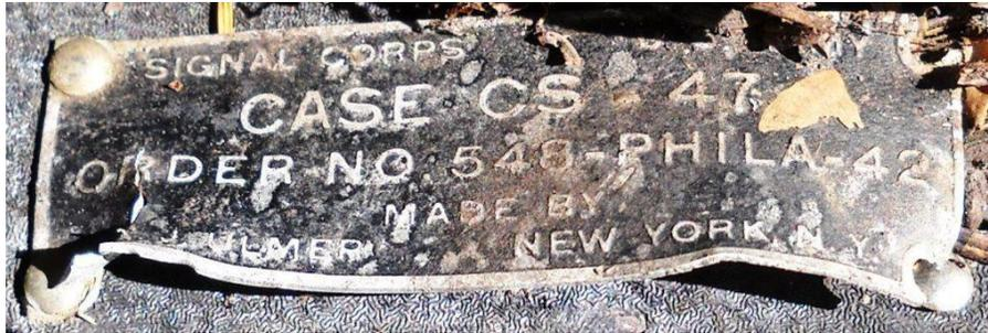
Several Beech part numbers were found along with a couple of data tags. Found on one box was a data tag for the “CS-47” dated 1942. It was the case for the BC-230 Transmitter Coil Set, part of the SCR-183/283 radio, photo by Dave Trojan.
