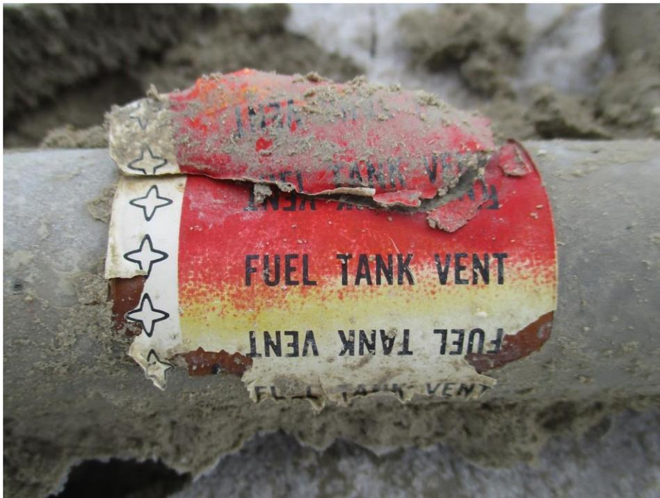
The label on this part is intact after sitting face down in the salt for 62 years
