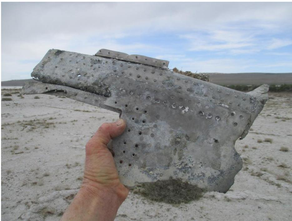
Lots of rivets in this layered sheet aluminum piece
