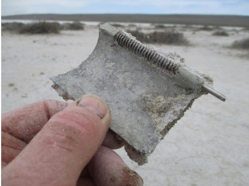
This curved piece has a spring-loaded hinge on it
