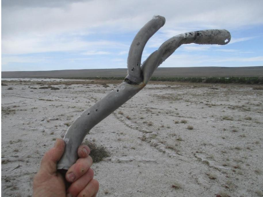
The holes in this aluminum tubing show how corrosive the salty soil is
