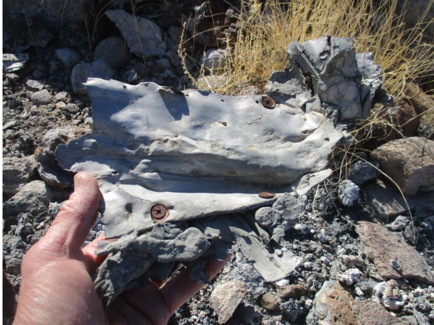
Melted aluminum at the B-17F impact site
