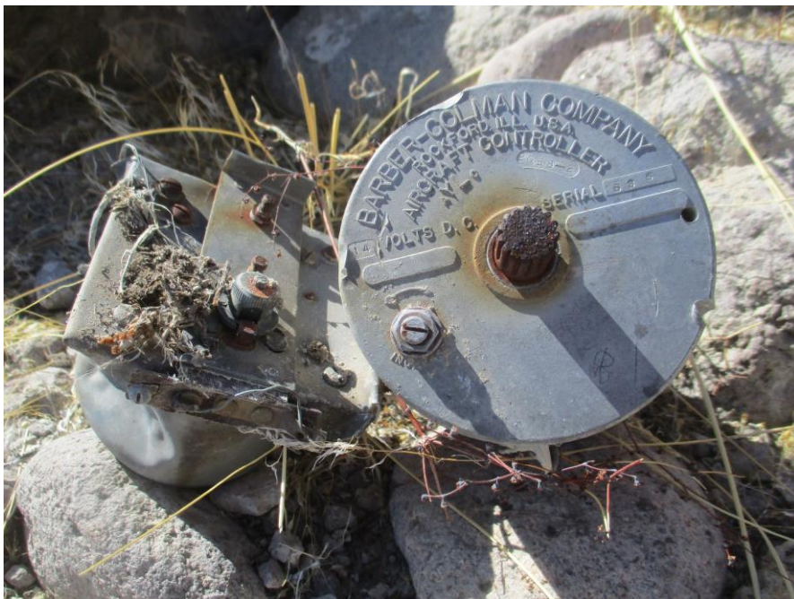
Electric servo used in radio-controlled aircraft
