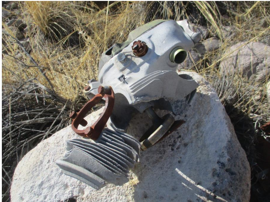
Part of a cylinder head from a Wright Cyclone R-1820 engine
