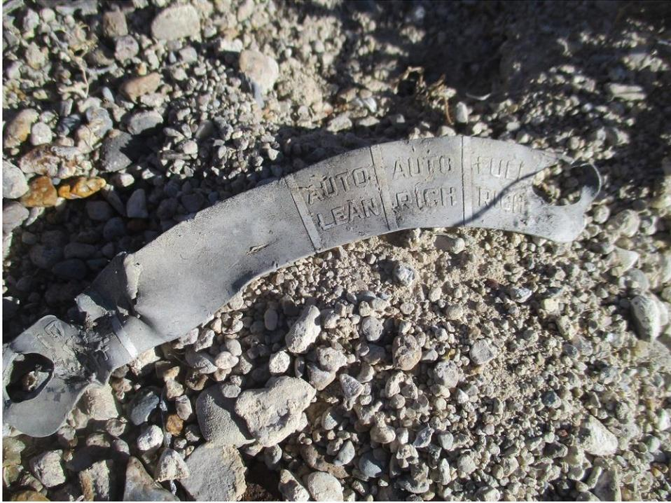
Placard from the mixture control lever in the cockpit
