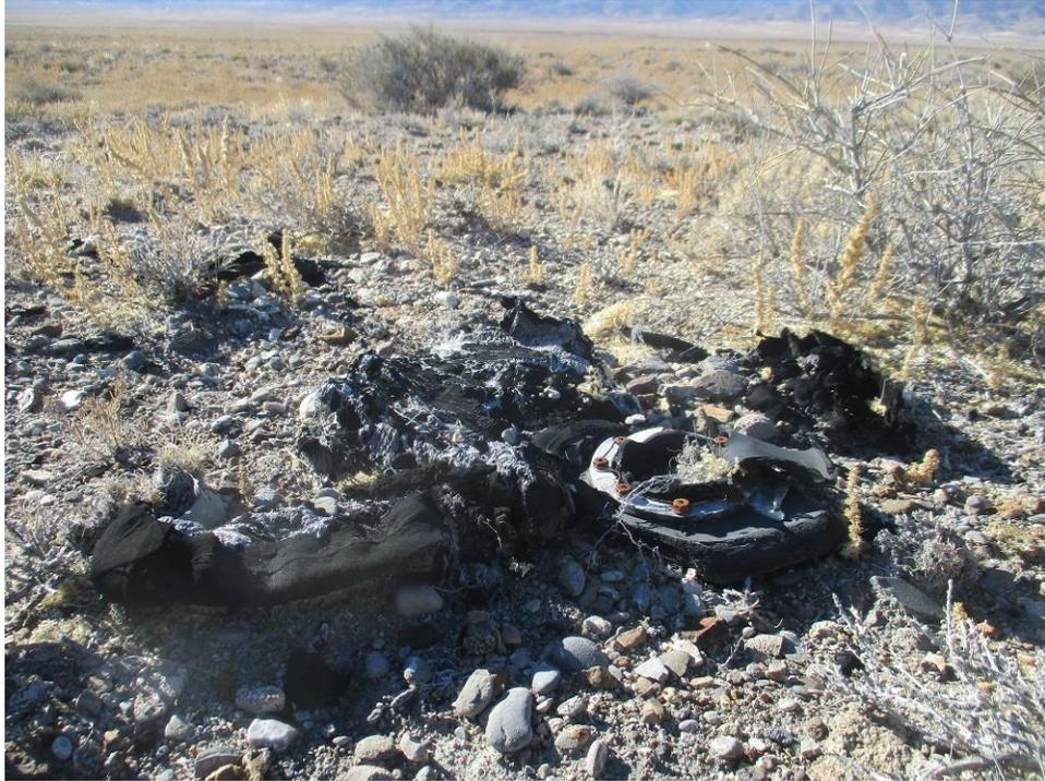
A rubber self-sealing fuel tank with filler opening at right
