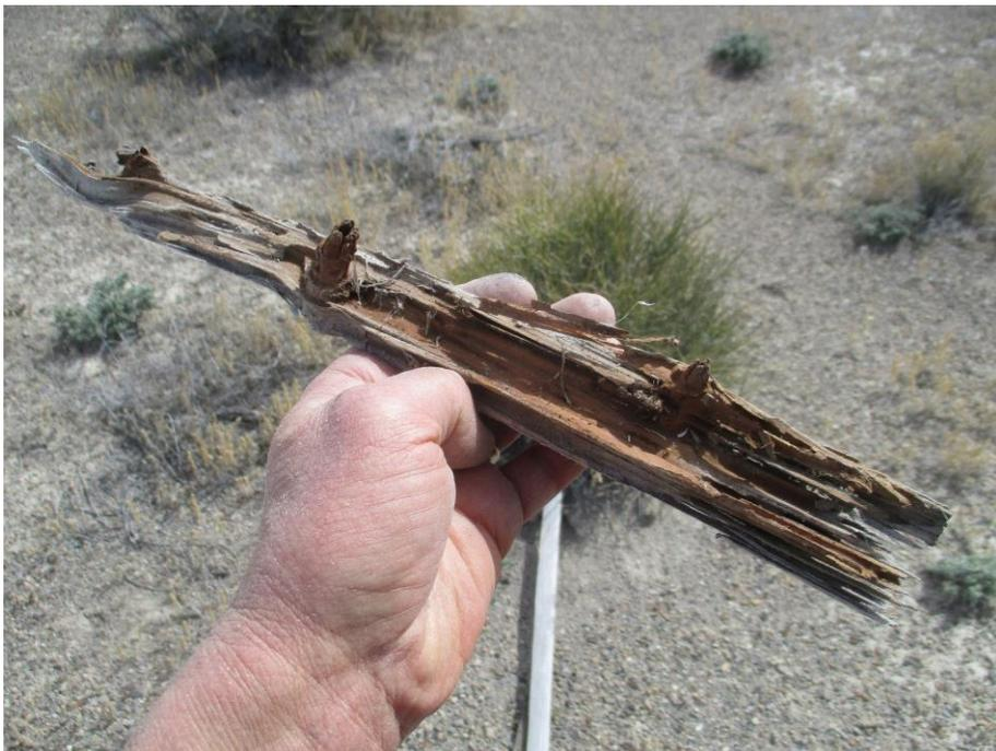
The aviation-type fasteners in this wood mean it was part of a wing
