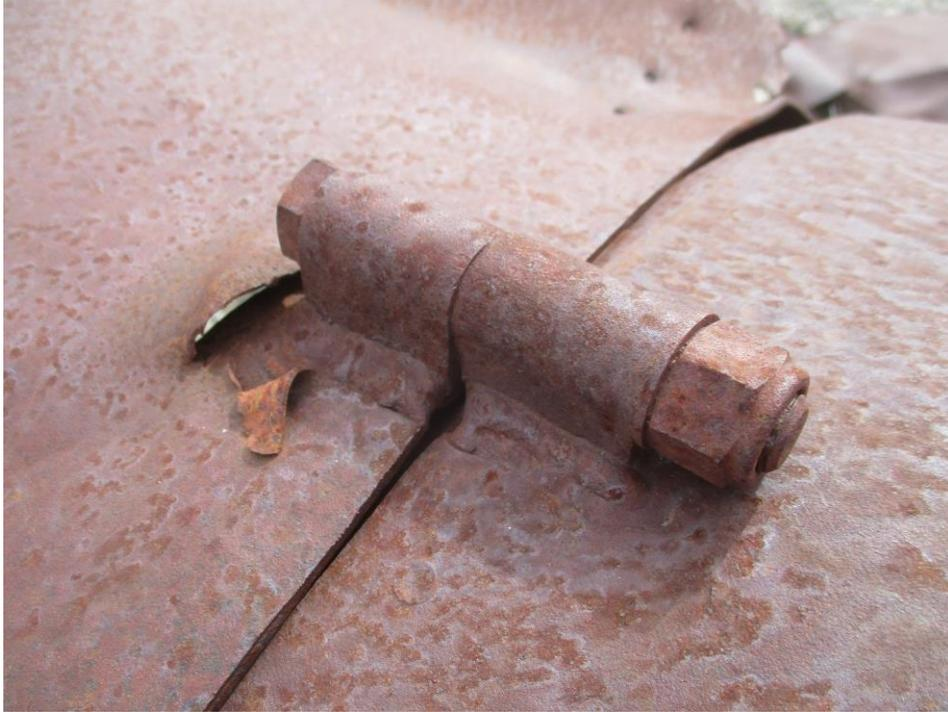
Large exterior bolts held the warhead to the fuel tank section
