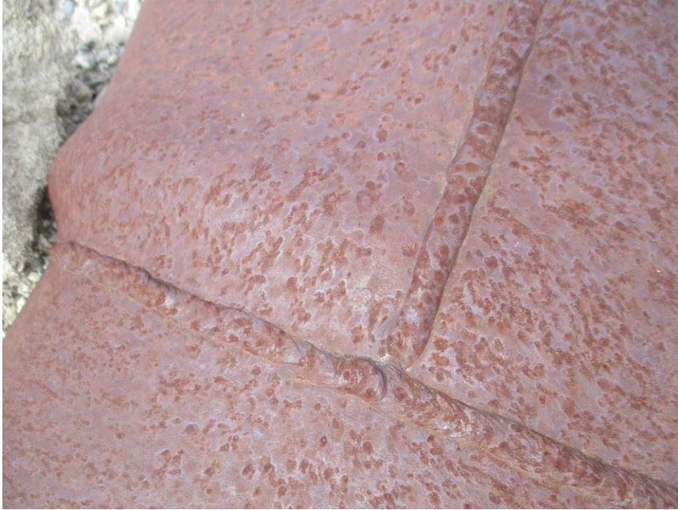
An example of the welded steel construction of the fuselage
