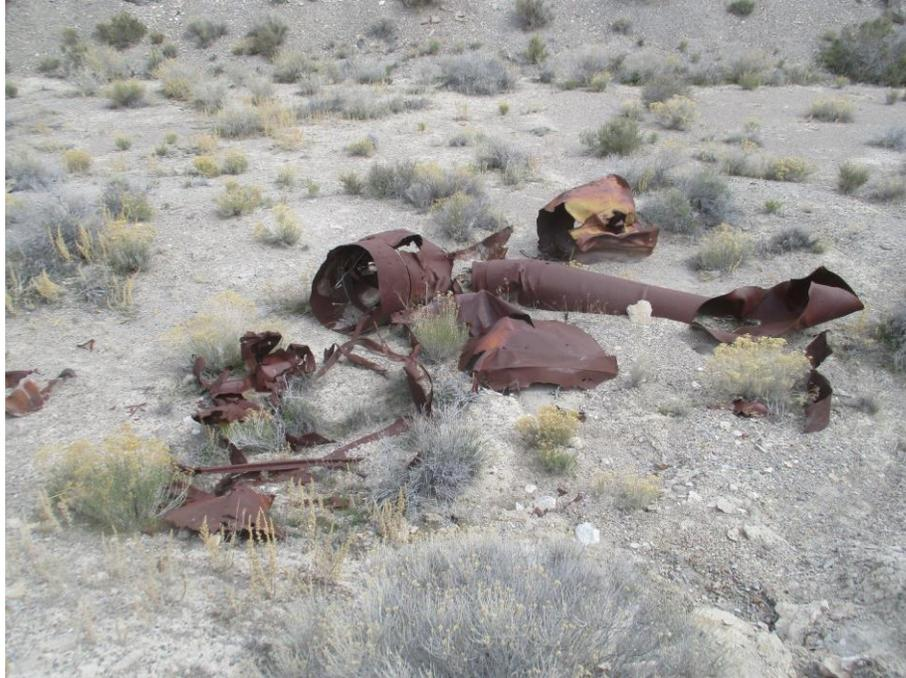
The warhead section is in the center, with the rear fuselage to the right and fuel tank above
