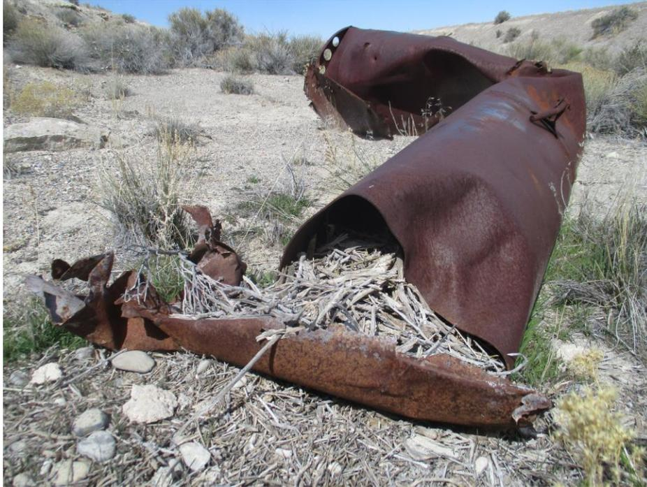
The tailpipe of the pulse-jet engine, which bent in half on impact
