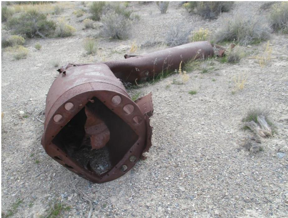
The intake of the pulse-jet engine, with intake shutters and fuel injectors missing
