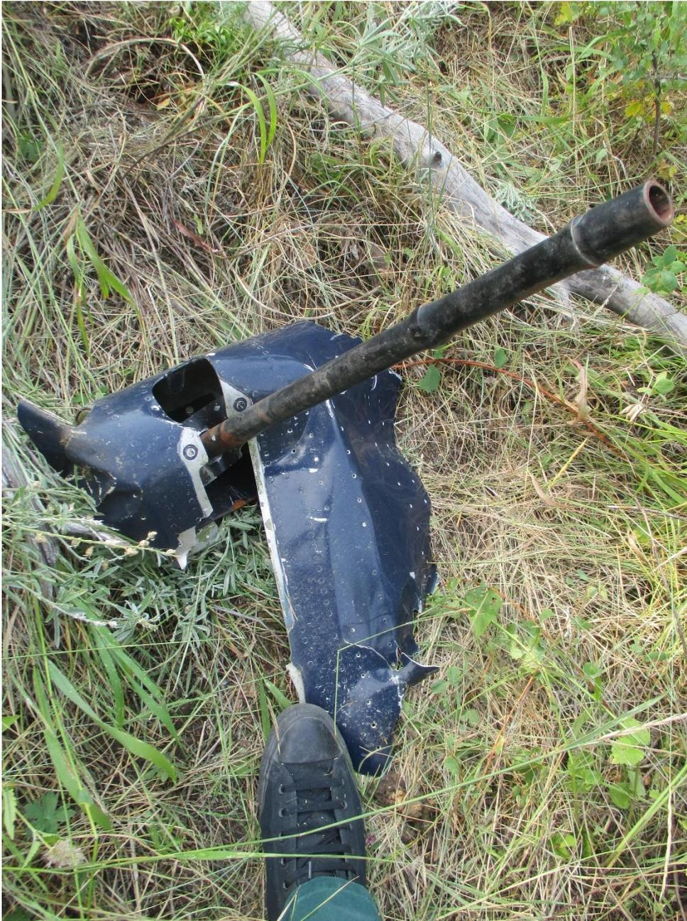
An imitation machine gun barrel fitted to the Skyraider after the original armament was removed
