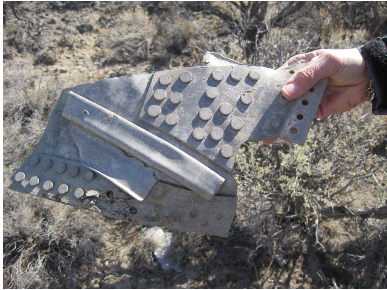
Several layers of riveted aluminum
