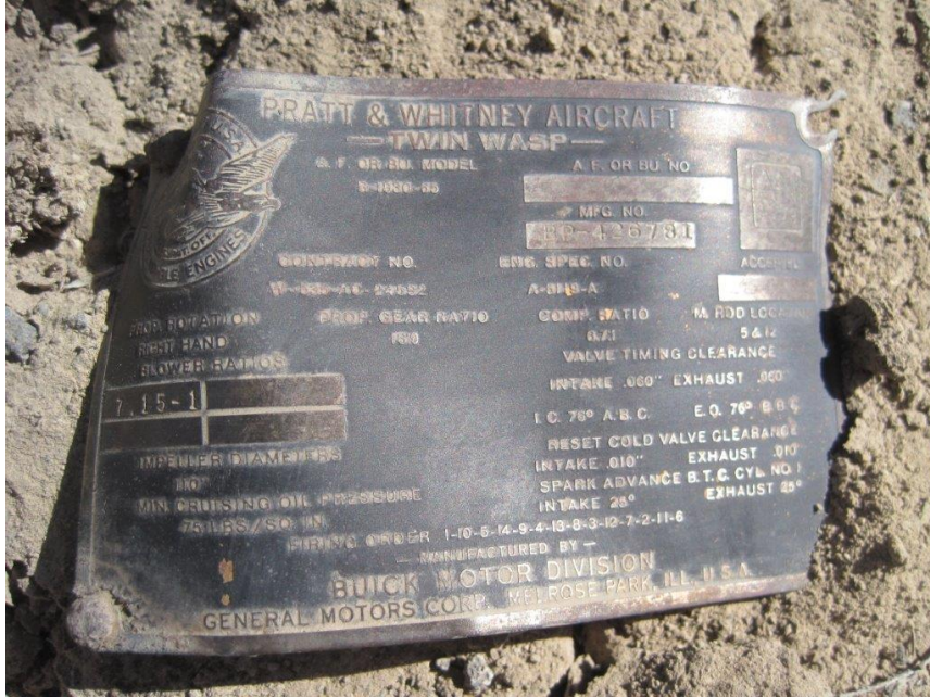
Data plate from a Pratt & Whitney R-1830 radial engine
