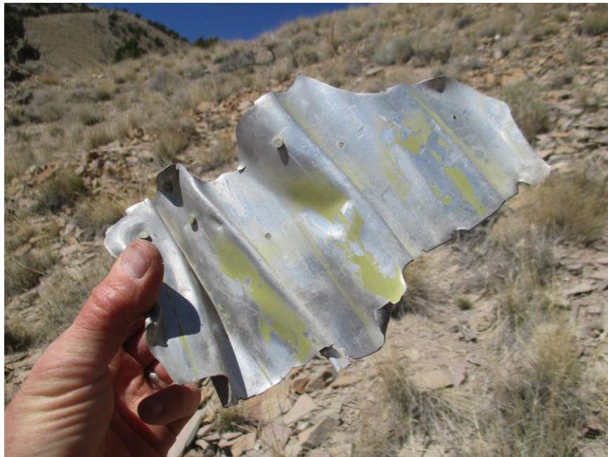
Green zinc chromate paint is still visible on this piece
