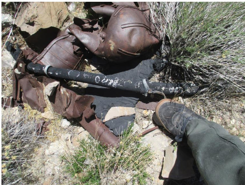
Crushed oxygen bottles and a large rubber hose
