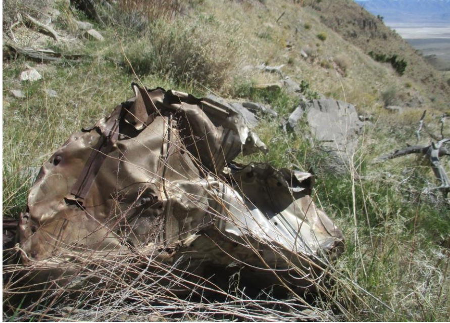
A stainless-steel engine firewall
