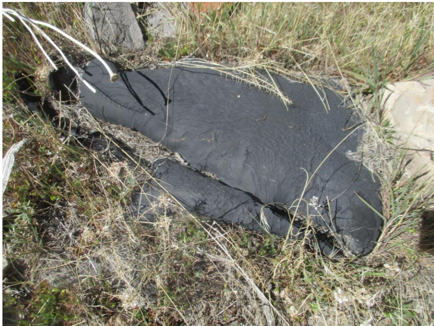
Rubber from a self-sealing fuel tank
