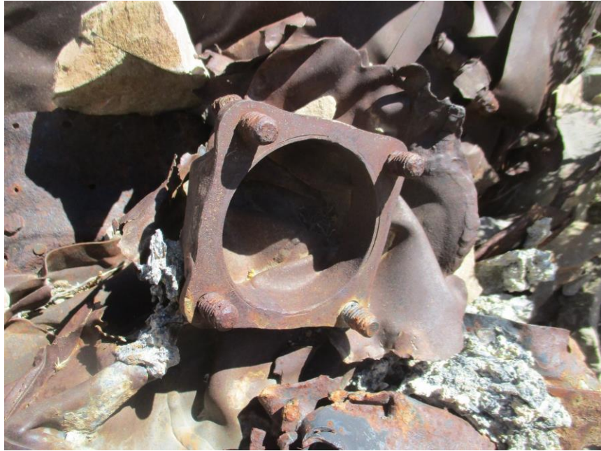
An exhaust pipe flange
