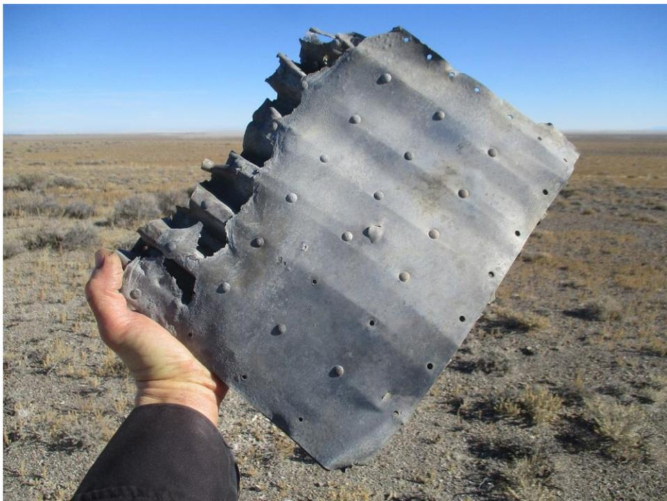
A riveted aluminum panel, possibly from a wing
