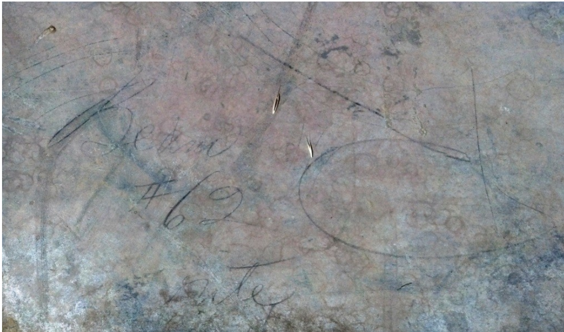
Manufacturing markings "Beam #62" found on part, photo by Dave Trojan
