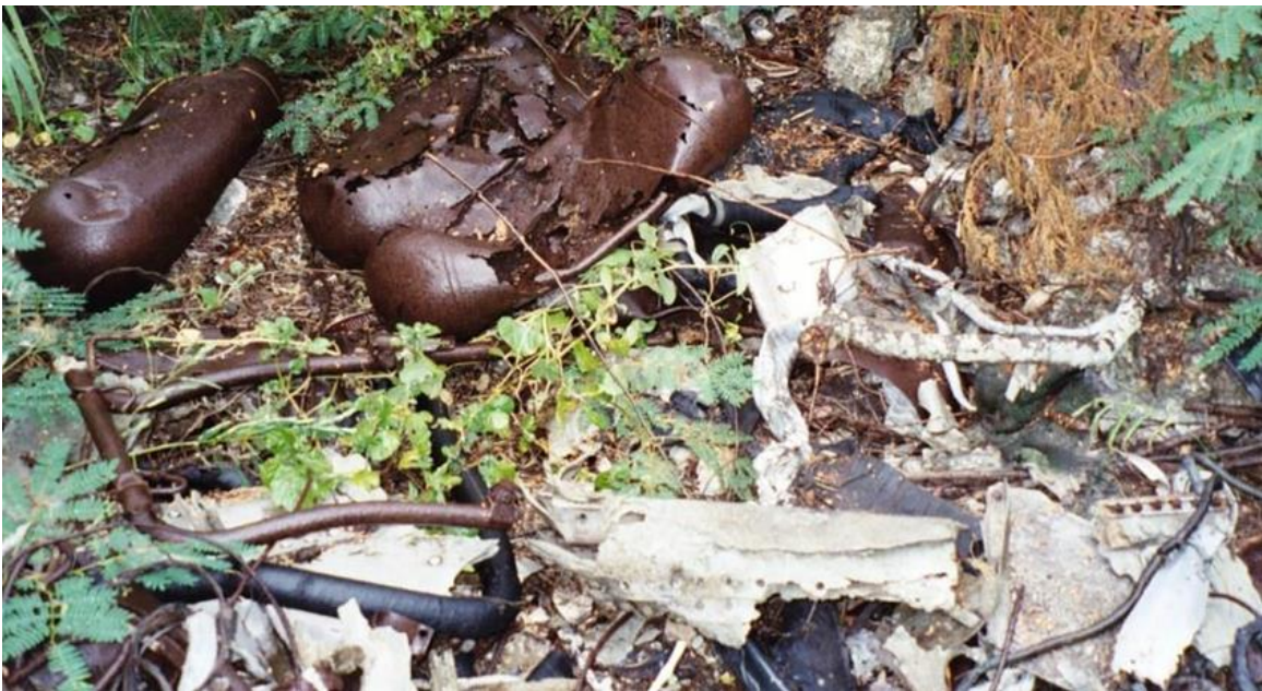
Three oxygen bottles and the pilots' armored seat back plate in the debris field bore witness to the three crewmembers that were aboard the ill-fated plane.
