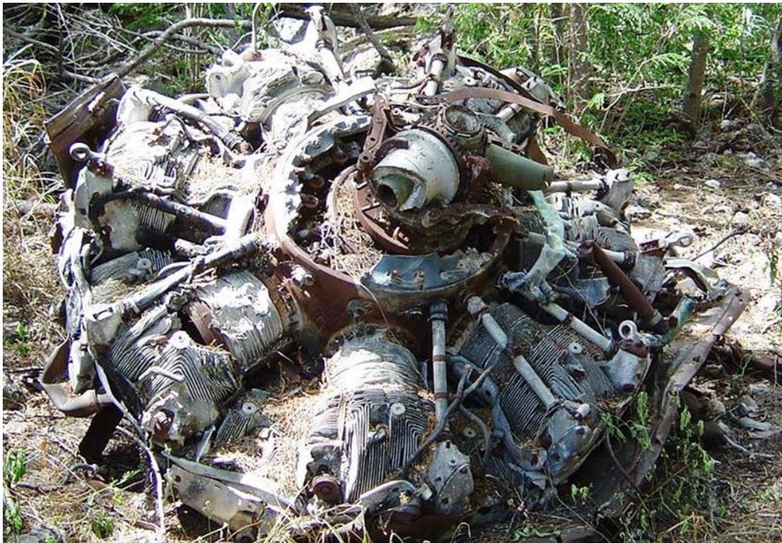
The most prominent feature of the crash site was the Wright R-2600-20 Cyclone 14-cylinder radial engine which lies on its back. You could see where its propeller blades were broken off from the impact of the accident.
