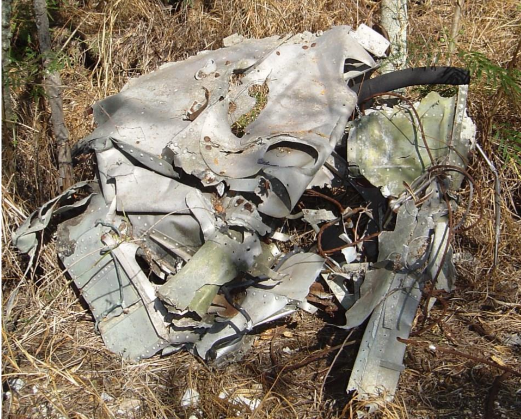
A wing fragment was identified by its access ports. It still had traces of the Navy blue paint with fuel lines and control cables hanging from it. Photo circa 2007
