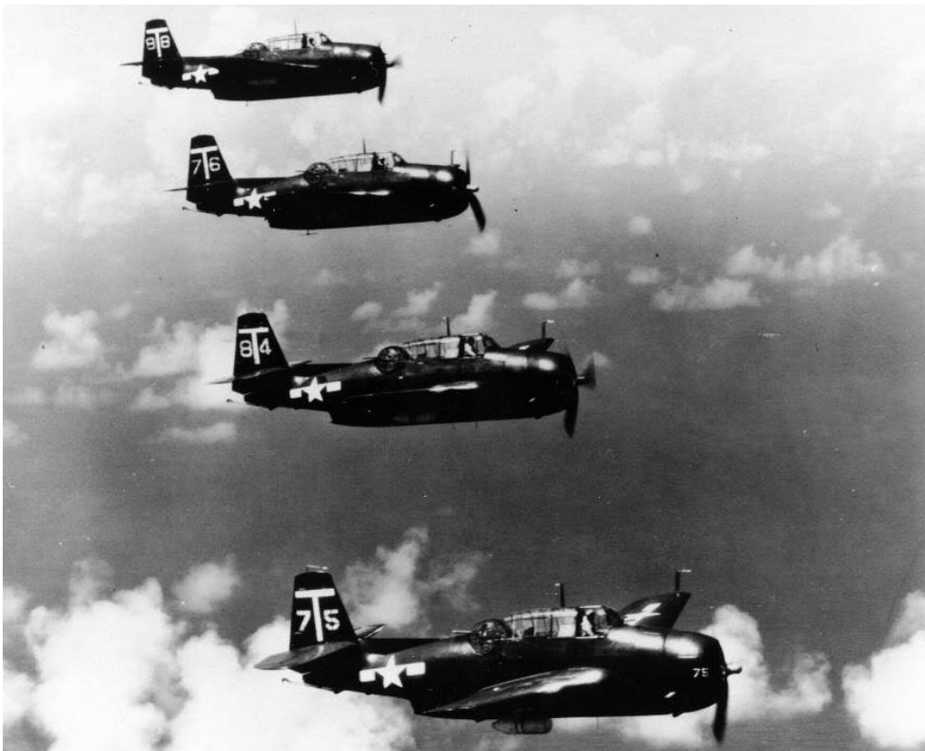
TBM-3Q Avengers from VA-2A USS Tarawa circa 1946; note the top two have the small twin-dipole DF antenna under the fuselage behind the bomb bay
