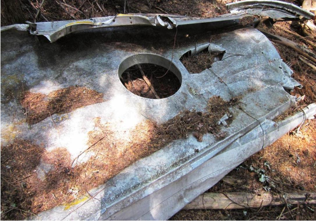
**This large piece is the floor of the aircraft. Both sides and the top of the fuselage were ripped off. A 35mm motion picture camera was mounted in the round hole to film each bomb run to record students bombing scores, photo by Sam Parker.**
