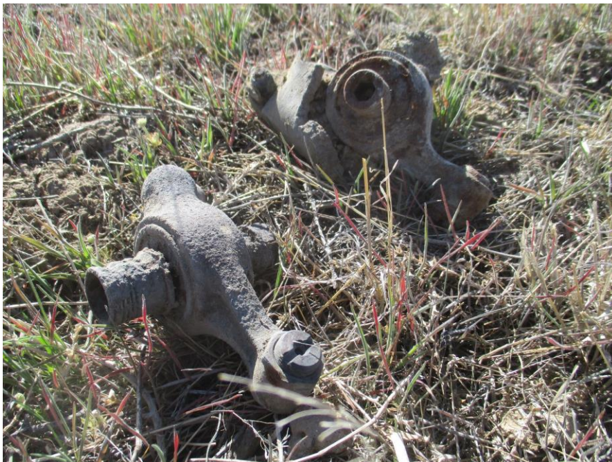
Two rocker arms from an engine
