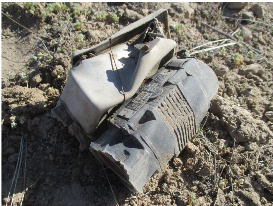
A Lear Avia electric motor used for opening and closing landing gear doors
