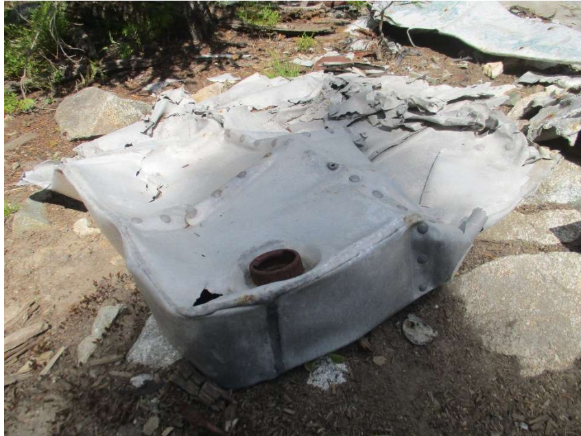
One of the fuel tanks located in the wings
