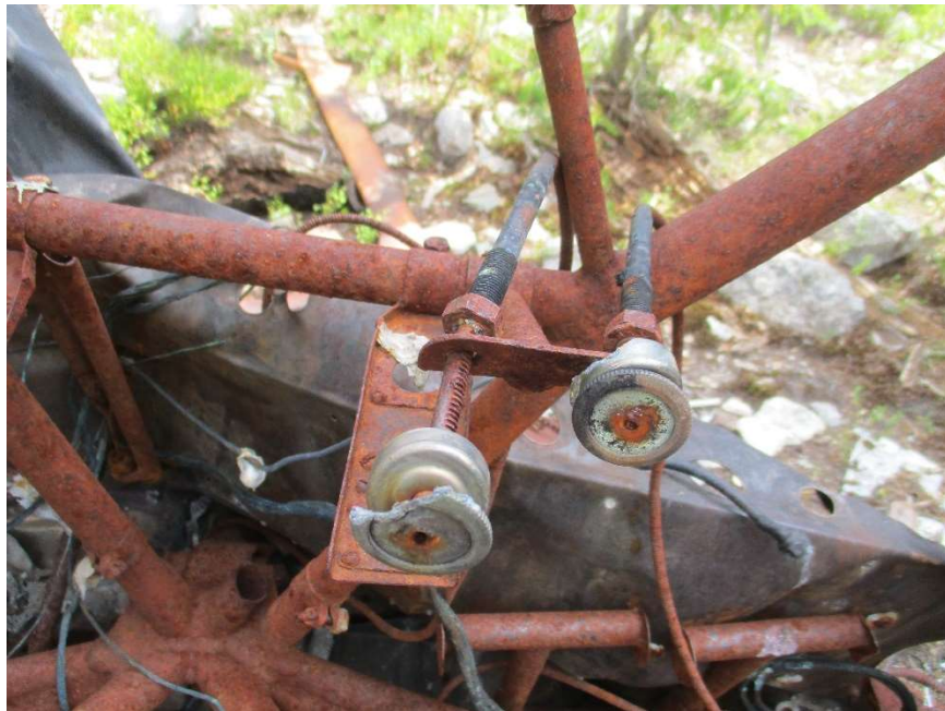
A pair of cockpit controls, with the co-pilot's rudder pedals visible at lower left
