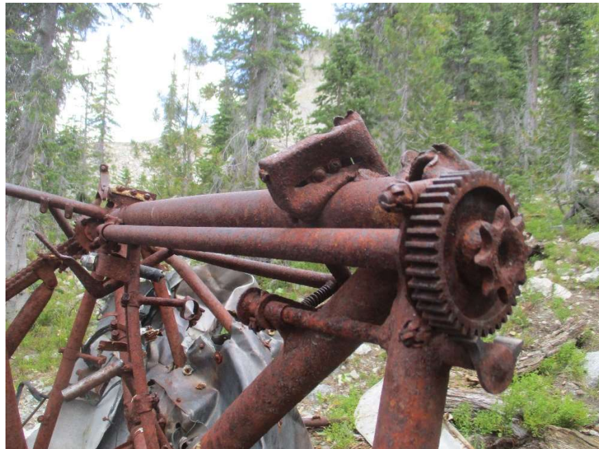
Sprockets, gears and chains associated with the cockpit controls
