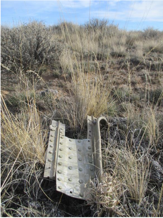
Riveted aluminum structure
