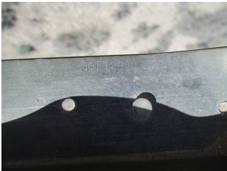
The "89" part number prefix means this is wreckage from a P-47
