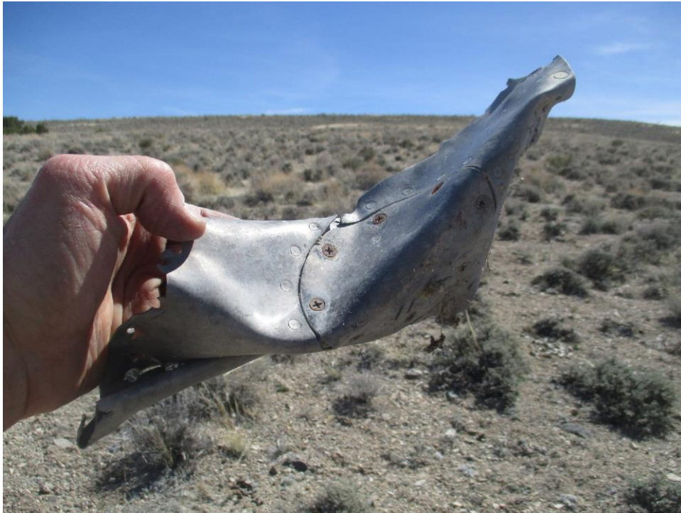
An inspection cover from one of the wings
