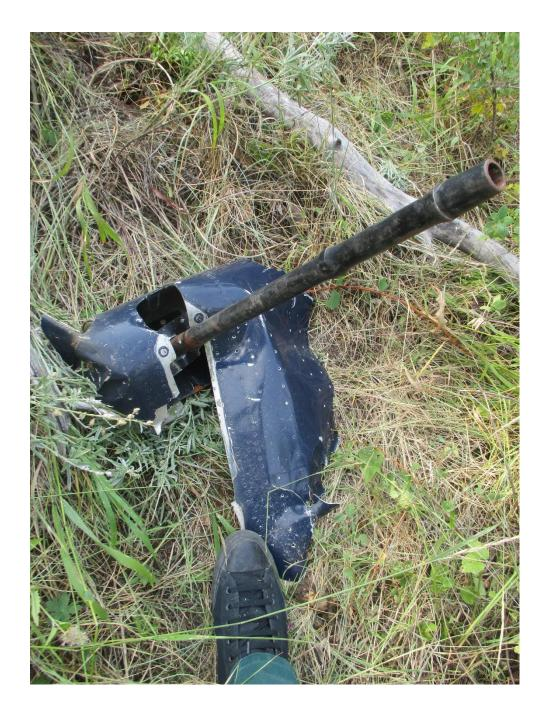
An imitation machine gun barrel fitted to the Skyraider after the original armament was removed
